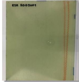
GRE Laminate (from 3Ax 1200 gsm)
