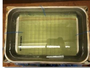
GRE Laminate immersed in recovery solution & Conditioned @ 80-90°C for 6 hrs.
