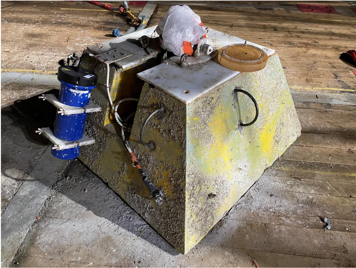
Figure 23: ADCP station fitted with an ROV compass
