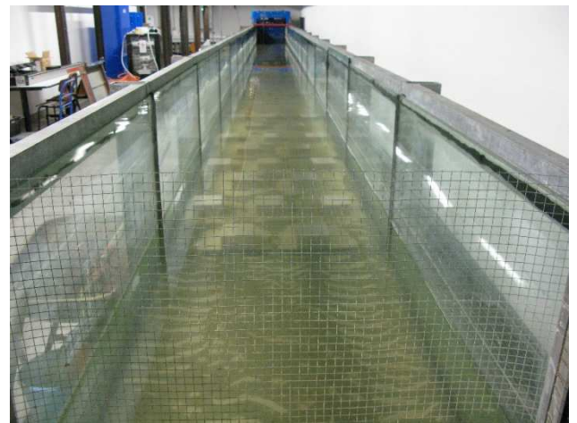
Figure 2: Turbulence-generating mesh and blocks installed in the LABIMA water channel.
