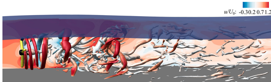
Figure 5 Instantaneous wake dynamics represented with Q-criterion iso-surfaces and contours of streamwise velocities, obtained from a LES using DOFAS (Ouro, Ramírez, et al., 2019)
