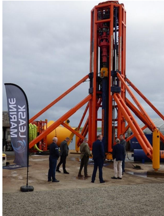
Figure 44 | LHS Swift anchor anchoring ROV and Leask Marine's subsea drilling rig
