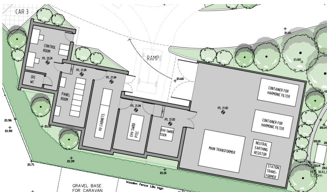
Figure 7 | Close-up of plan showing substation layout
