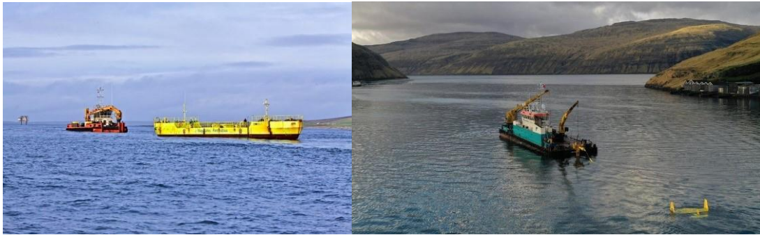
Figure 39 | Medium work boats for marine operations: ATIR install (left), Deep Green install (right)
