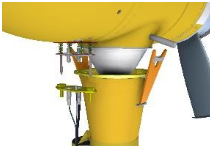
Figure 28: 3D view of a passive wet mate connection (SABELLA)
