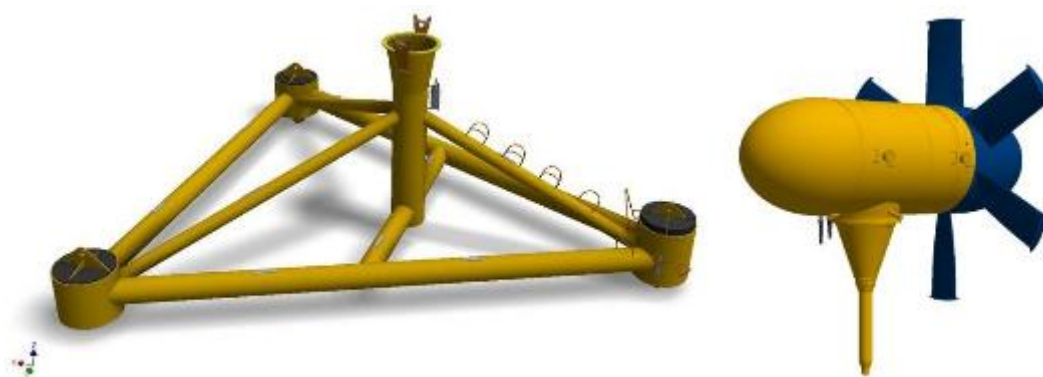
Figure 6: Base and turbine of the "Sabella D10" tidal turbine (SABELLA)
