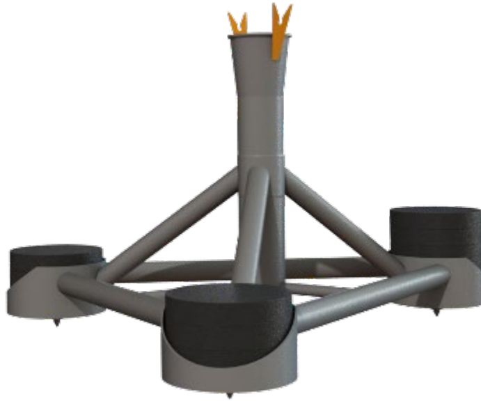
Figure 27: 3D view of the preliminary design of the D08 base (SABELLA)
