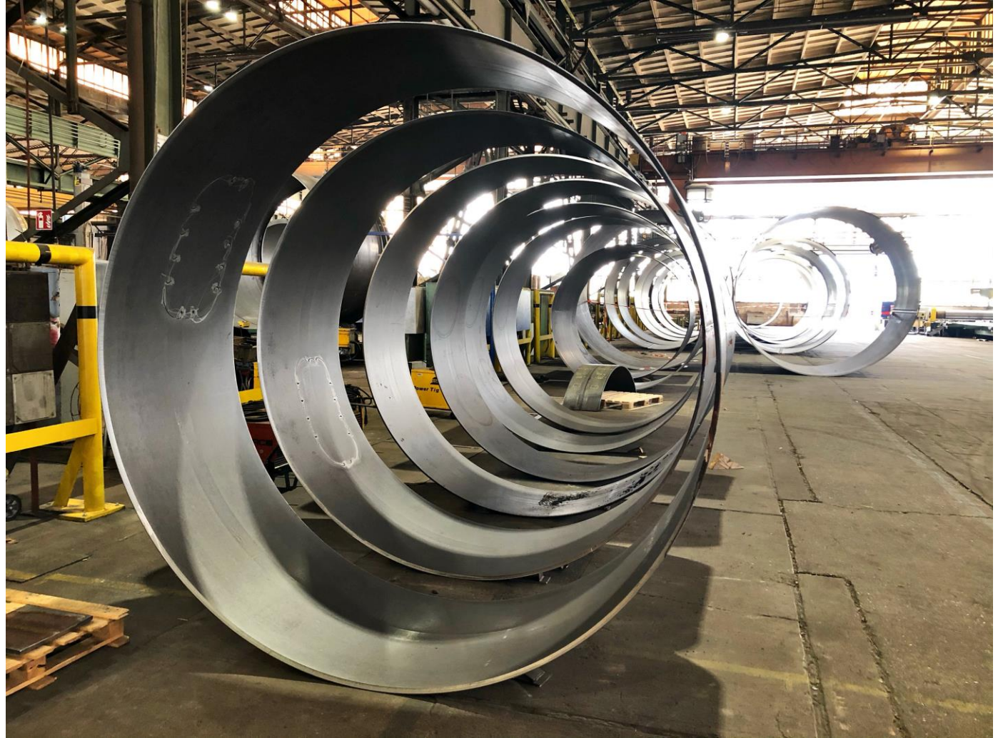
Nacelle cylinder segments
