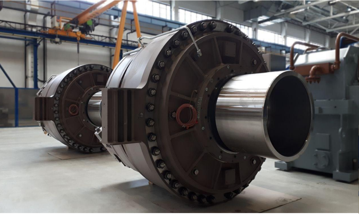
Gearboxes completed testing and awaiting painting at Wikov in Czech republic
