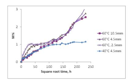
Different thicknesses, infused & preg, aged in natural seawater at 25, 40 and 60°C
