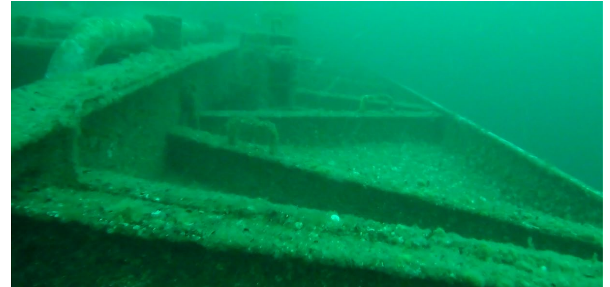
Parts with no anti-fouling coating – After 16 month
