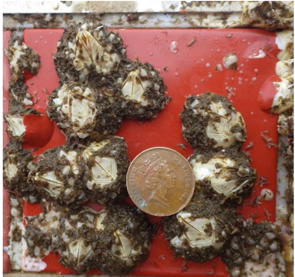
Chirona hameri on FRC coating after 24 months
